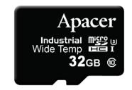
The MicroSD 5.1 card comes with 8-pin interface, designed to operate at maximum operating frequency of 50MHz or 100MHz. It can alternate communication protocol between the SD mode and SPI mode and is backward compatible with SD 2.0 devices. It performs data error detection and correction with very low power consumption.
